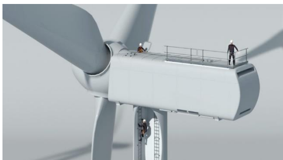
Figure 16: Turbine with guardrails [12]
